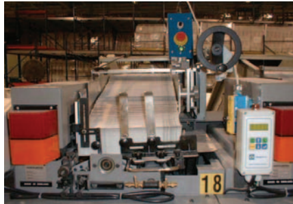
Note the well jogged, low pile height control. Good jog quality with the full range of signatures and gimmicks.
