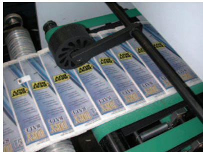
Tab inserted on signature in the shingled stream at exact count
